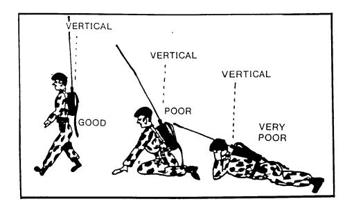
Figure B If Operating Ground Wave Best Results Should Be Obtained With the Whip (vertical) and Use of a Dangling Ground Plane Enhancement Tail
